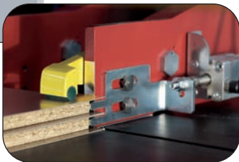
Automatic formatting device for overlay material
