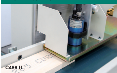
C486-U Water-based printer for the classification of sized pieces
