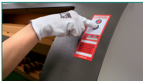
Servo-actuated thickness adjustment
