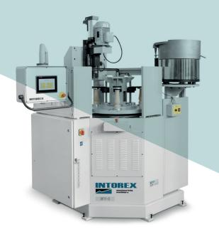
A specially designed boring and inserting machine to fit screws and bushes into sofa legs, feet etc. The standard machine is equipped with a bottom boring unit, a screw inserting and manual feeding unit (screws M8x70). On request a vibration bowel with automatic feed can be specified. Work cycle of the machine is programmed electronically with the rotary table having 3 work cycles:
