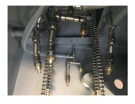
The operating mechanisms (chains, pulleys, bearings and wheels) are all located in a liquid-proof area completely outside the impregnating chamber protecting them by the typical corrosion due to treatment liquid.
