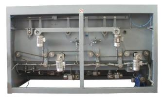
A powerful fan unit providing up to 600 lt/min assures the required quantity of air to the 5 blowers.
