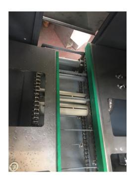
The workpiece feeding system is made of a serie of V type metal bracket mounted on a gardle chain running inside the machine. The V shape assures a minimum contact (2 points only) between the workpiece and the feeding unit. Furthermore two polizene adjustable guides ensure a constant and safe motion of the workpieces
