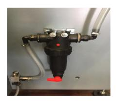
The 8 spray nozzles are fan-shaped type to grant a perfect and homogeneous primer application. Thanks to a quick removing mechanism nozzles cleaning and maintenance is extremly simple. A series of filters prevent the nozzles block due to the primer waste or the dust particles. For an optimal liquide dosage, each single nozzle is equipped with an independent regulator.
