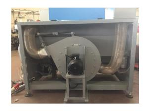
Thanks to 5 air blades any excess of primer is litterally blown away from the work-piece with a super grade of finishing including profiles with narrow angles or special profiled shaped. The 5 air blades are located on adjustable arms that permit the best position according to the workpiece dimensions
