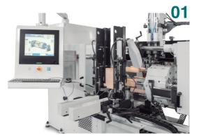
Standard machine: Frontal hopper feed loader, one CNC roughing unit, two CNC copiers (roughing and finishing), two sanding copiers and one sanding unit with oscillating brushes with cut cloth abrasive. Detail of machining a sofa leg.
