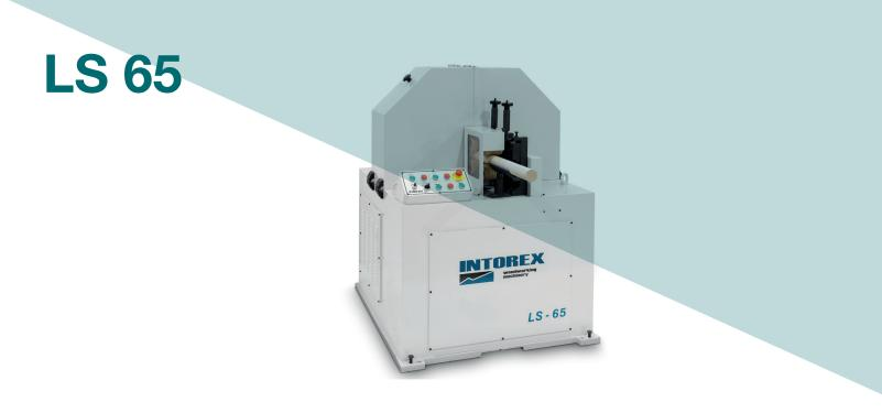
A dedicated through feed automatic machine for sanding round bars for diameters ranging from 15 to 65 mm. The machine is equipped with 2 x sanding belts which are in rotation over the piece to be sanded. The workpiece length can be unlimited and feeding is by 4 infeed/4 outfeed drive rollers of adjustable speed from 8 to 25 mm/min and can sand components such as brooms handles, agricultural tools handles, umbrellas, stair rails among others.
