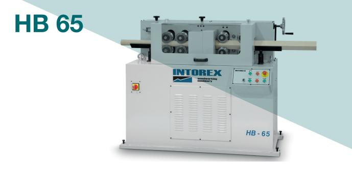
A dedicated machine to produce rounded bars from square section material. Finished diameters range from 15 to 65 mm. The workpiece length can be unlimited and feeding is by 4 infeed/4 outfeed drive rollers of adjustable speed from 8 to 25 mm/min and can manufacture brooms handles, agricultural tools handles, umbrellas, stair rails among others.
