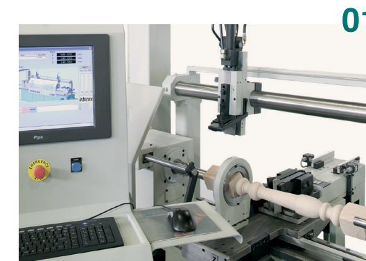
Standard machine: 2 CNC copiers, centering unit and 2 automatic back knife units.
