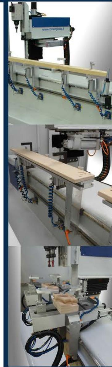
Sectioned bench, standard version, with rotating lockings.
