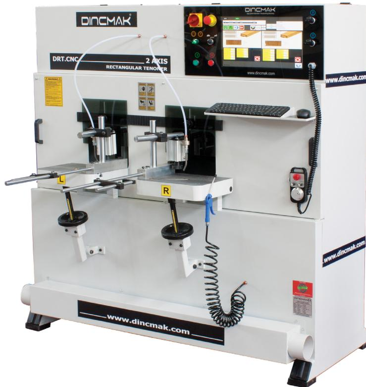
**A simple to use, extremely flexible twin table machine for producing precise, high quality round end tenons, square end tenons or dowels for solid wood furniture**
